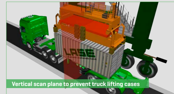
Function principle - gap detection by 2D scan plane
