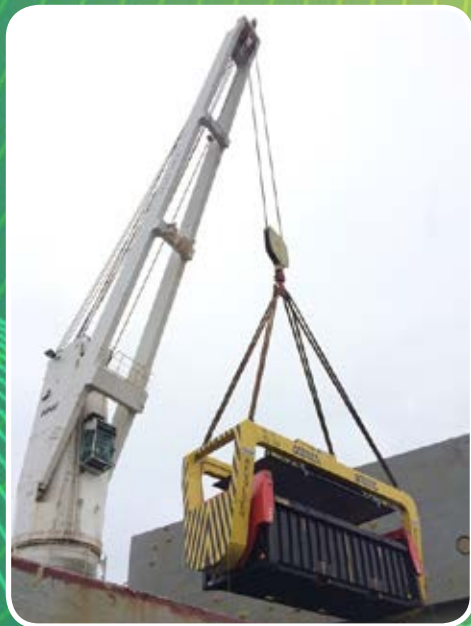
Patented lid lifter replacing the container lids.
