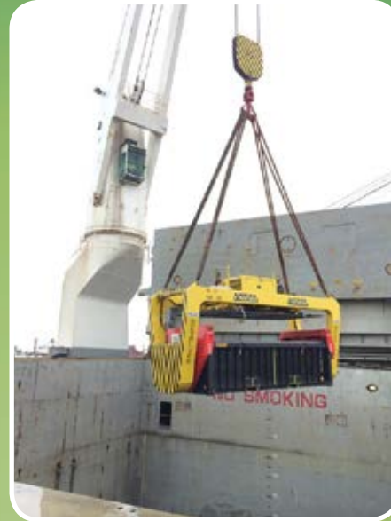
Patented lid lifter in use.
