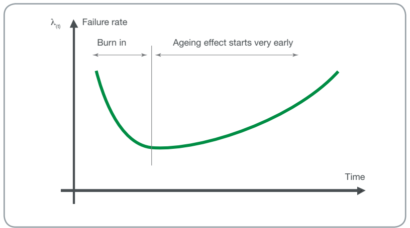
Fig.16 - Mechanical component failure rate over time.
