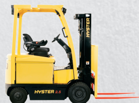
E2.2KN, E2.5KN, E3.0KN, E3.2KN, E3.5KN 2 200-3 500 KG @ 500 MM Compact design and cushion tyres ideal for indoor applications
