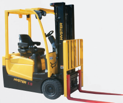
A1.3XNT, A1.5XNT 1 300-1 500 KG @ 500 MM Streamlined design with 3 wheel configuration
