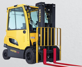
J2.2KN, J2.5KN, J3.0KN, J3.5KN 2 200-3 500 KG @ 500 MM AC drive and hoist motors with customizable performance settings
