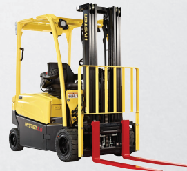
J1.6KN, J1.8KN, J2.0KN 1 600-2 000 KG @ 500 MM Streamlined design with 4 wheel configuration
